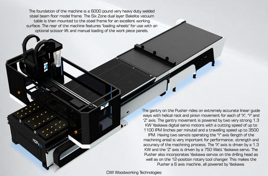
The gantry and working areas of the machine are surrounded by a safety cabinet with emergency stops on all four sides of the machine. Each of the spindles use automatic dust hoods with 6" hoses to a main 8" dust collection inlet above the machine. There are pneumatically controlled connections to the drill head, router spindle and pusher bar for cleaning the table surface.
