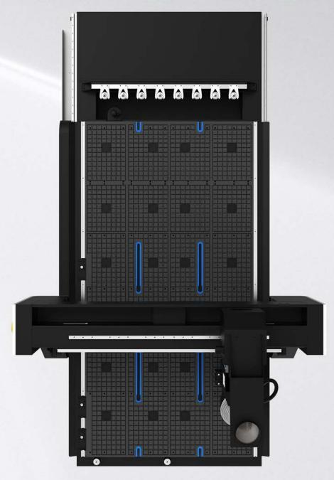
The CabinetMaker CNC offers 12" of "Z" travel while providing up to 10.5" of machining height which is extremely helpful for the occasional solid wood machining most shops encounter.
