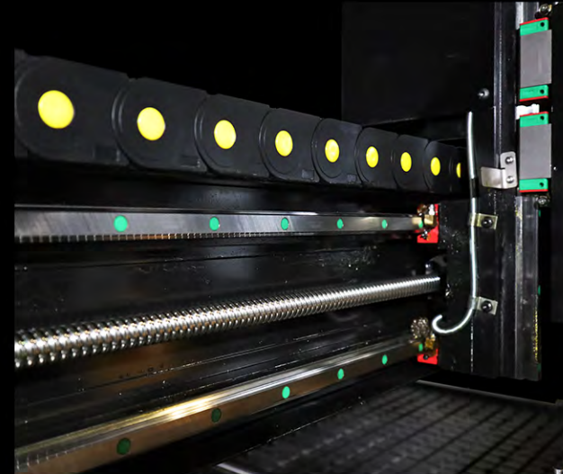
THK Linear guides rails on all 3 axis
